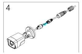
Connect the plug terminal to the RJ45 jack.
