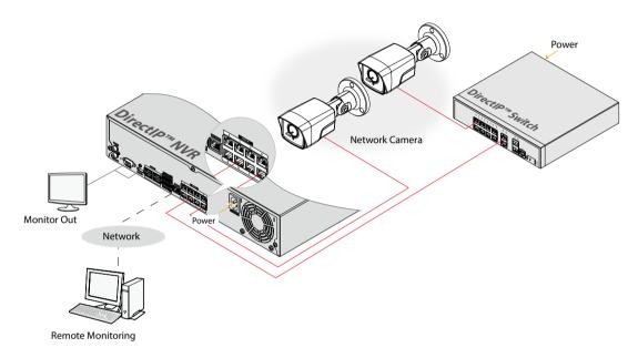
DirectIP<sup>TM</sup> NVR makes it easy to use cameras without extra network configurations. Each camera can be controlled via the DirectIP<sup>TM</sup> NVR setup menu, without any PC. For detailed camera settings, please see the camera setting pages of DirectIP<sup>TM</sup> NVR manual.
