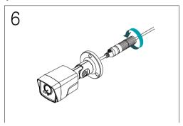
Lock the waterproof cap into the waterproof cap body.
